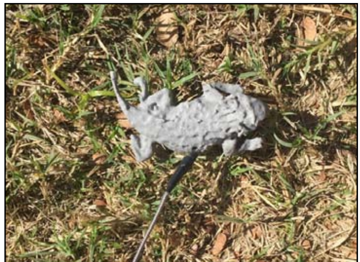
3d printed ABS horned lizard attached to the Arduino-based thermal coupler used to measure microhabitat thermal spectrum. (Photo by Marcus Thibodeau)
