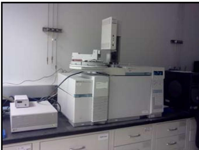
Organochlorine pesticides were analyzed using the gas chromatograph-mass spectrometer (GC-MS).
