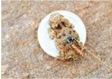
“Old diode” - A Texas horned lizard hatchling with the initial reflector design that included copper wire and a diode (lizard is sitting on a quarter coin)
