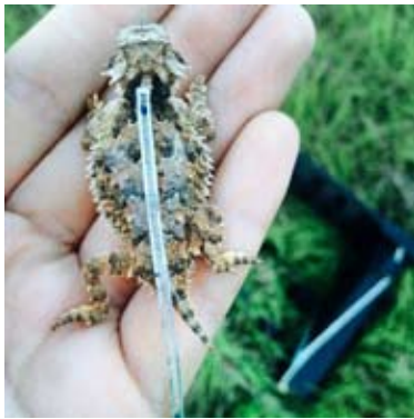
“New diode” - A juvenile horned lizard with the most current reflector design that allows for detection distances up to 5m away.
